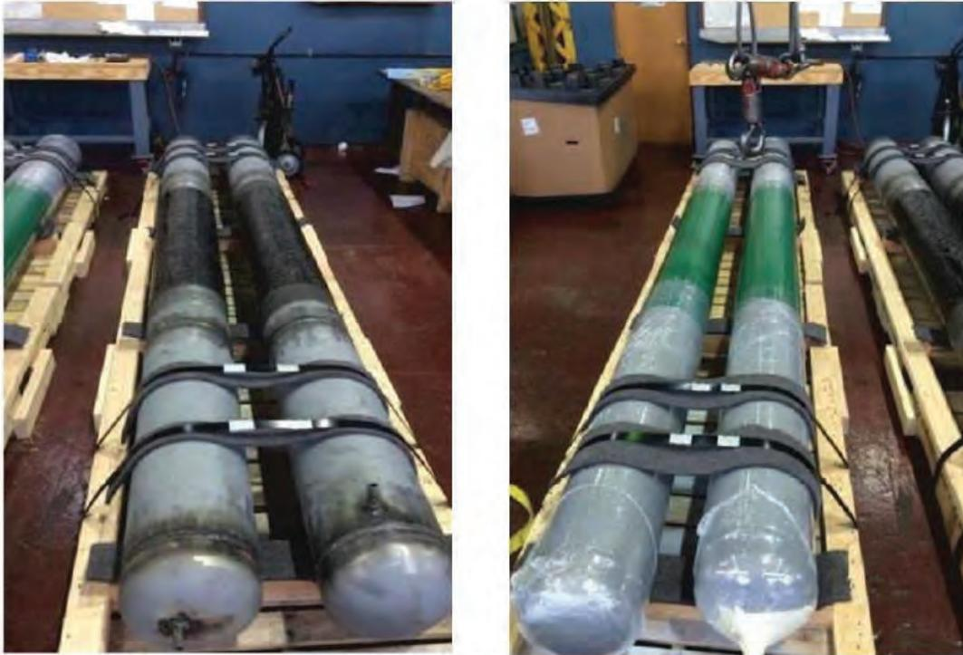
*Figure 3. Bitumastic coated (left) and green tape (right) pipe samples.*
