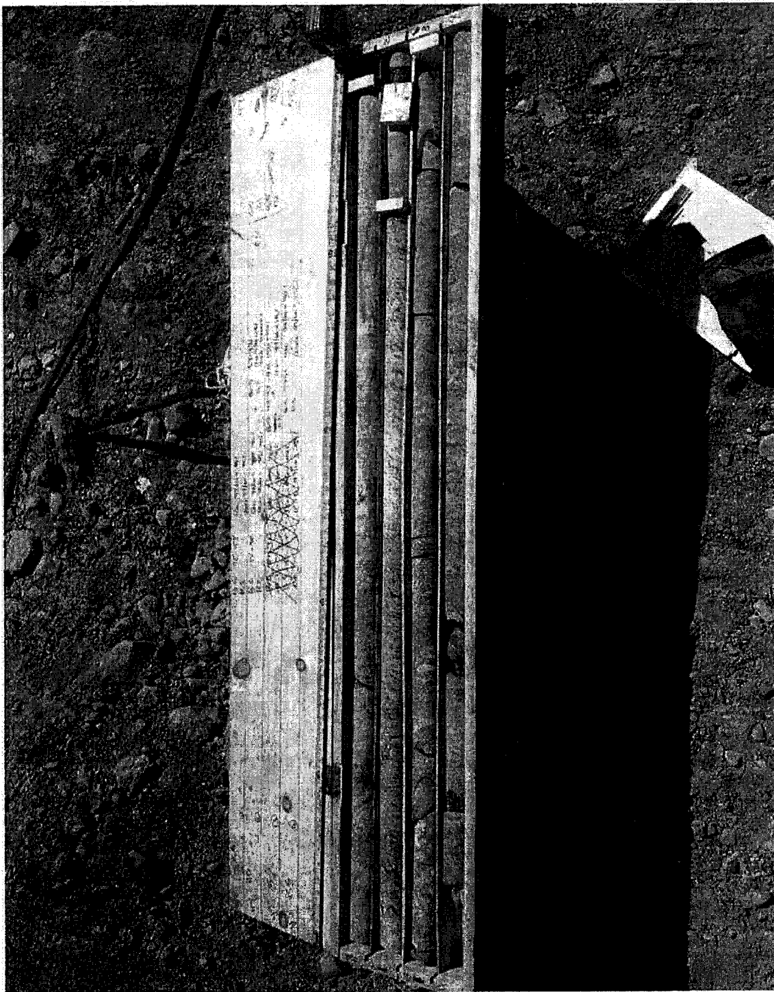
PHOTO 3: Rock Cores from Boring B-6 (Top 2 core runs in box) and Boring B-5 (Bottom 2 core runs in box)
