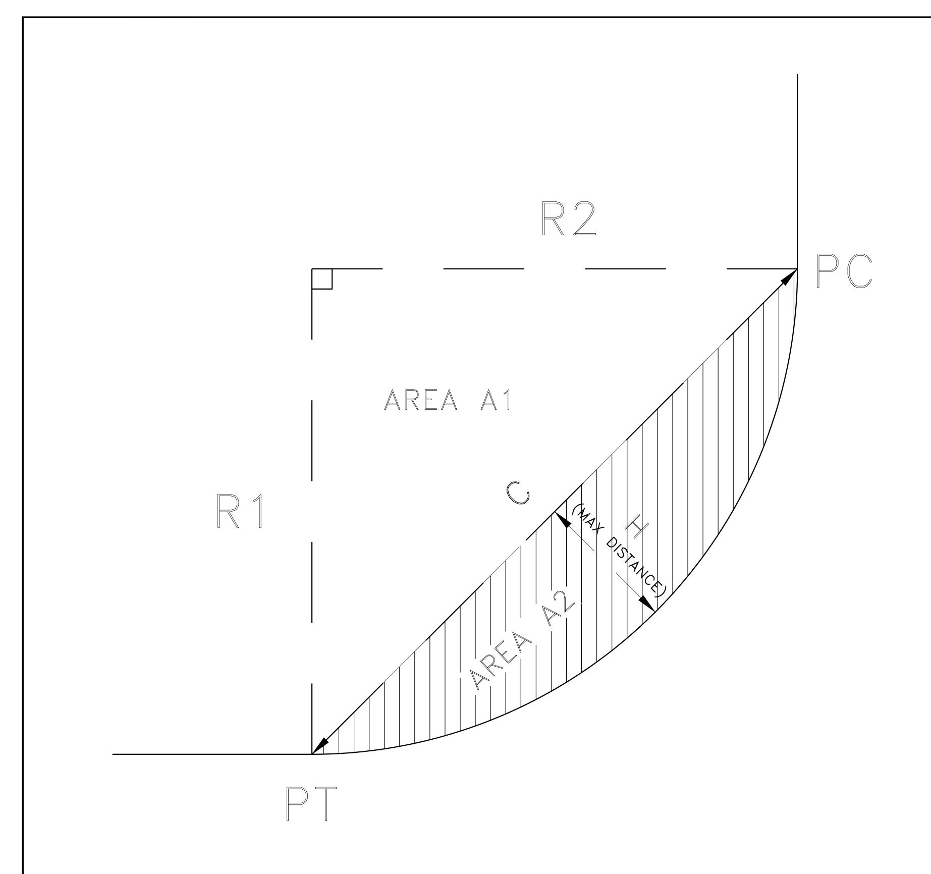
PLAN VIEW OF 7" SIDEWALK FOR CORNER QUADRANT (N.T.S.)
