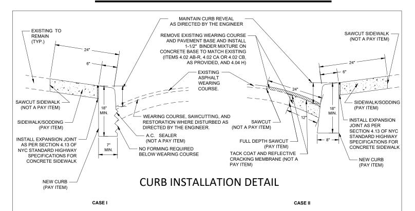
CASE I TO BE USED FOR AREAS WITH CONCRETE PAVEMENT, INCLUDING REINFORCED CONCRETE BUS STOPS. ANY CONCRETE PAVEMENT DAMAGED BY THE CONTRACTOR MUST BE RESTORED AT NO COST TO THE CITY.
