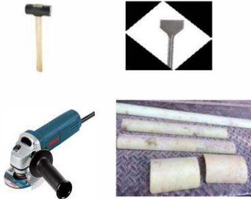
3 lb. Hammer, 2" chisel, Rotary Cutting Tool & Blade, Micarta protective "half moon"
