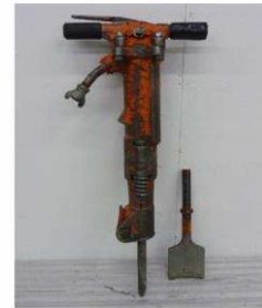
Never use a jackhammer to break out ducts, or use in the vicinity of a gas main or service.
