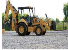
Never use a backhoe Bucket, or ramhoe attachment by electric of gas facilities
